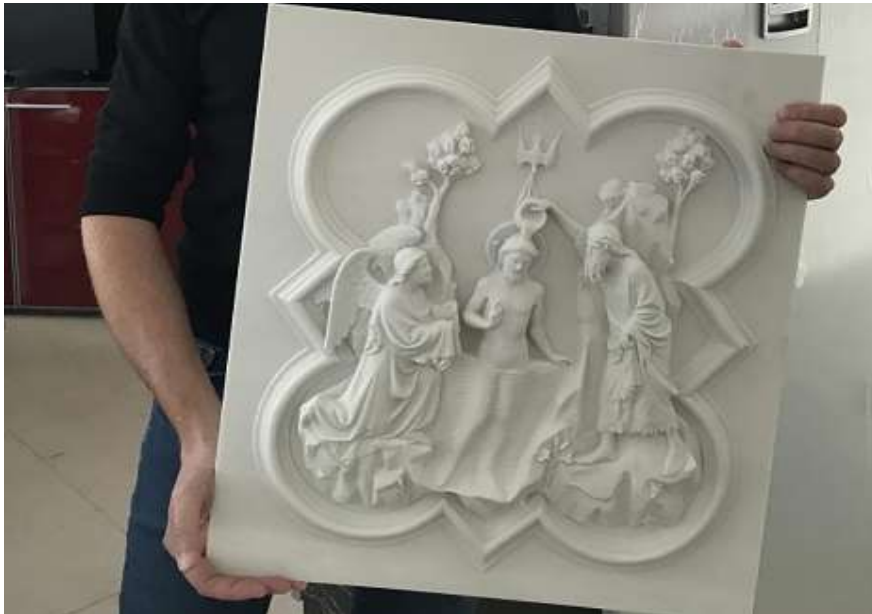
Figura 10: Painel das portas históricas impresso na impressora 3D. Fonte: Bringing an Italian 14th century bronze masterpiece back to life with Artec | Artec 3D Scanners Applications (acesso em 11/09/2022).
