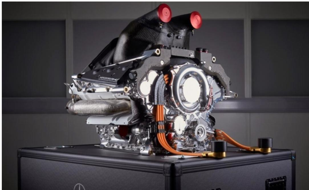
Figura 11: Motor V6 1.6 Litros Turbo – Mercedes-AMG.
