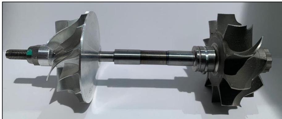
Figura 14 - Conjunto turbocompressor Master Power R474
