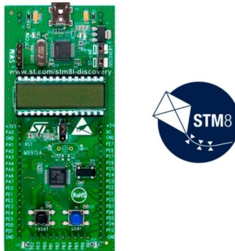
Figura 6 – Módulo STM8L Discovery. Fonte: (STMICROELECTRONICS, 2019).
