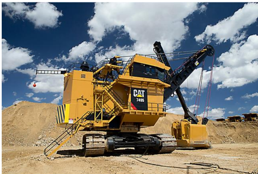
Figure 15 - Escavadeira a cabo Caterpillar 7495
