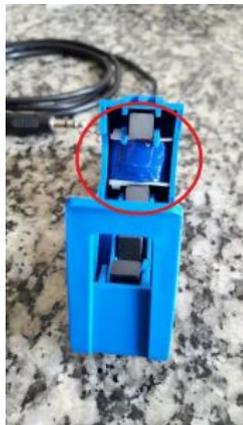
Figura 17 – Bobina interna do sensor SCT-013.
