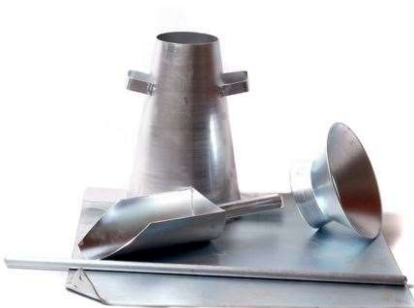
Figura 11: Conjunto Slump Test (Bombear, 2016)
